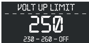
Picture 5. High voltage protection
