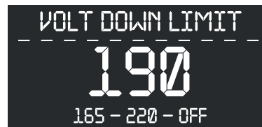
Picture 6. Low voltage protection
